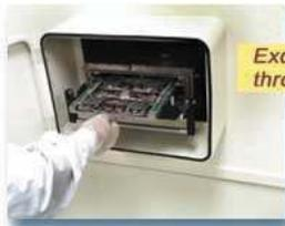
Exchanging the prober module through the airlock
