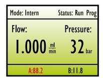
After the pump reached its flow rate, it automatically goes to HOLD; this means the pump is running, but the gradient program time is on hold.
