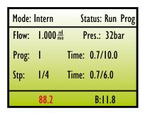
The bottom line shows the current gradient composition while the center of the status screen shows the current step, step time and total time.
