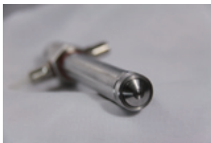
自动通针喷头 Automatic online nozzle cleaning
