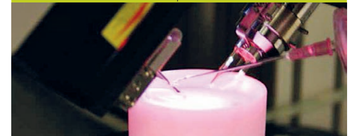
Light guide enables measurements at liquid/liquid interfaces and solid/liquid interfaces at variable angles between 40° and 72°
