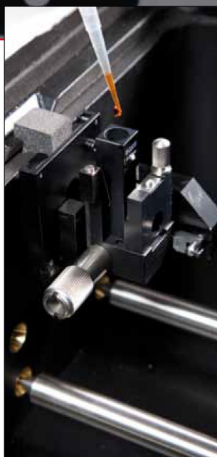
Autosampler for particularly high sample throughput
