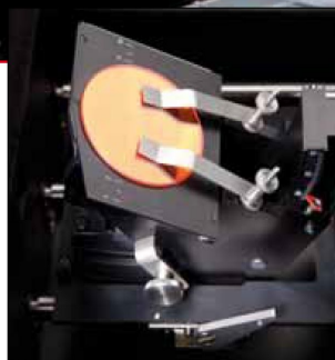
Reflectance attachment with variable angle for determining the refractive index and the film thickness
