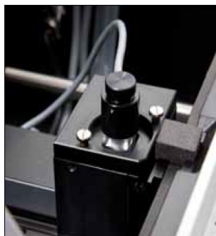
The peltier temperature controlled cell holder guarantees high temperature accuracies; the temperature is measured directly in the cell.
