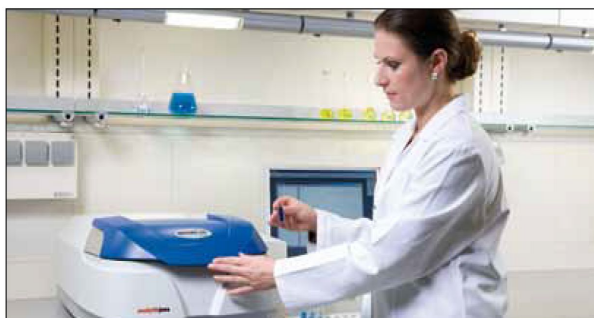
High sample throughput with the 15-cell changer or individual analysis with the single cell holder, the SPECORD® PLUS offers the ideal equipment for all requirements.
