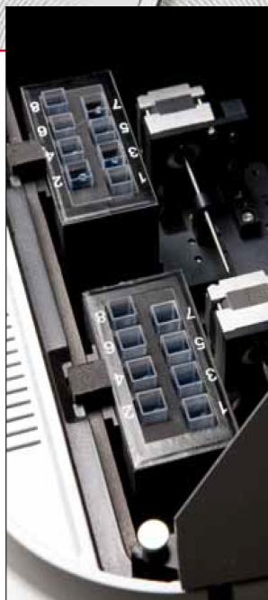
Double 8-cell changer for a speedy and an efficient working process
