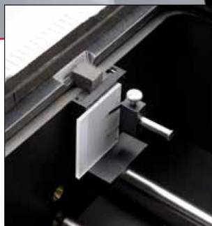
Solid sample holder to determine transmission characteristics
