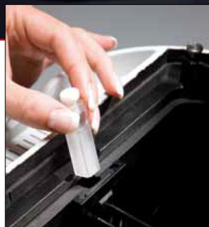
Position for turbid samples for measuring highly scattering samples
