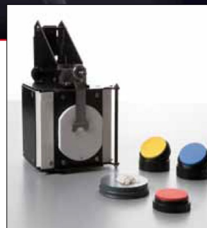
Integrating sphere for transmittance and diffuse reflectance measurements
