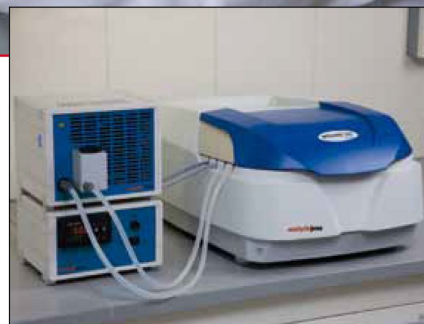
Peltier temperature controlled 8-cell changer performing measurements with high temperature accuracy
