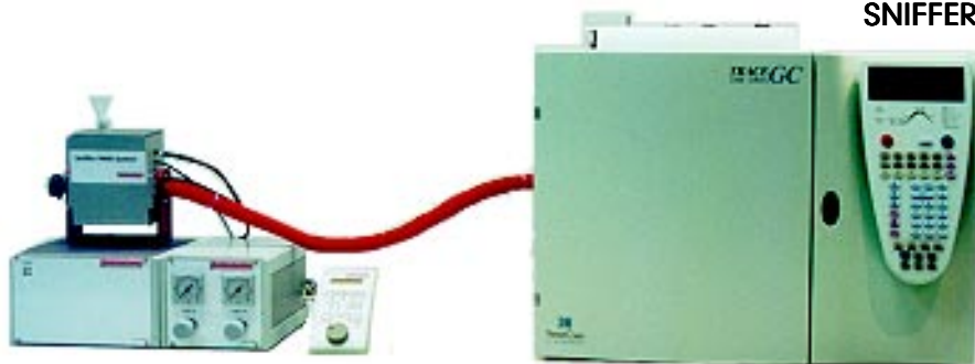
Complete GC-O system with trace GC
