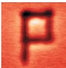
Figure 13. Magnetic lithography. Letter "P" is written by magnetic tip in continuous CoPt film with perpendicular anisotropy by similar way as shown in Figure 12.
