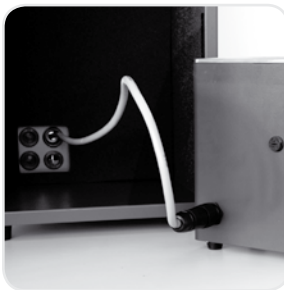
5. Connect the instrument cable to the waterbath and place into the sound-proof box.
