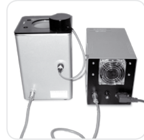
2. Connect the waterbath and control unit using the control unit cable.
