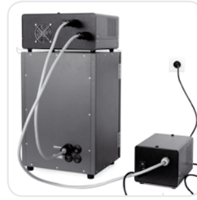
2. Connect the controller to the waterbath through the sound-proof box.
