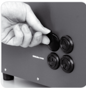
3. Remove the rubber cap from the back of the sound-proof box and feed the instrument cable through the upper left hole marked instrument cable.
