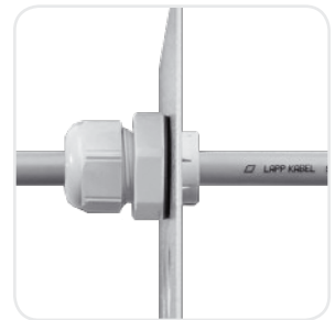
4. The fitting will secure the cable to the sound-proof box. Turn the front section counterclockwise to seal. Be sure there is enough slack in the cable.
