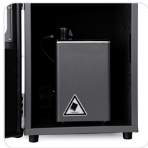
5. Connect the instrument cable to the waterbath and place into the sound-proof box.
