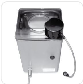
3. Connect the rotor. Rotate the black cap to secure the connection.
