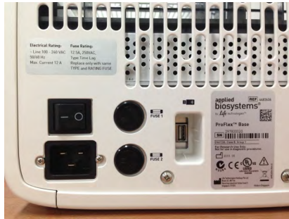
Figure 41 Location of the safety label on the rear panel of the ProFlex™ System
