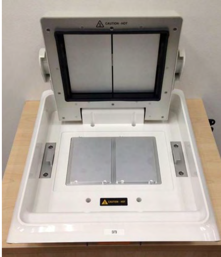
Figure 45 Location of the safety label on the ProFlex™ Dual Flat Sample Block
