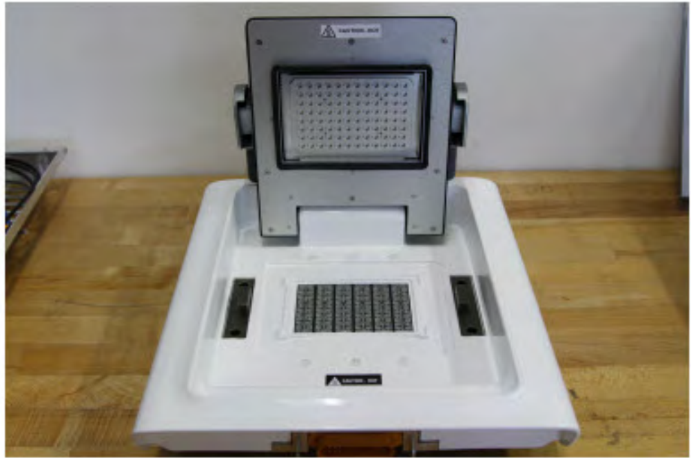
Figure 43 Location of the safety label on the ProFlex™ System 96-Well Sample Block
