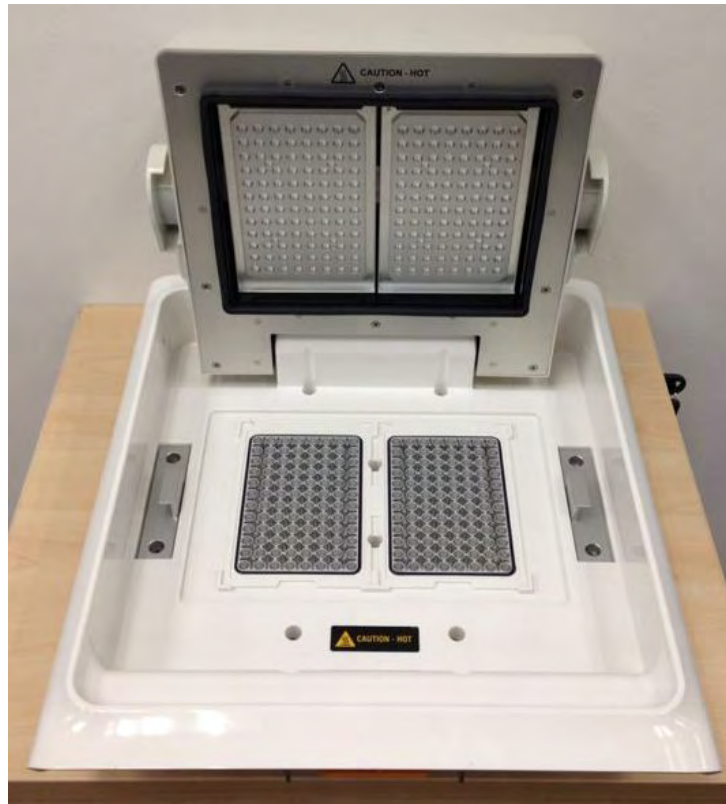
Figure 44 Location of the safety label on the ProFlex™ Dual 96-Well Sample Block
