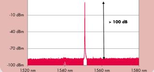
Yenista's unique T100 cavity eliminates the broadband spontaneous emission (SSE) that is normally present in an external cavity laser's output. The T100R has the lowest figure of merit for SSE of any tunable laser on the market and gives a dramatic improvement in a measurement's dynamic range.
