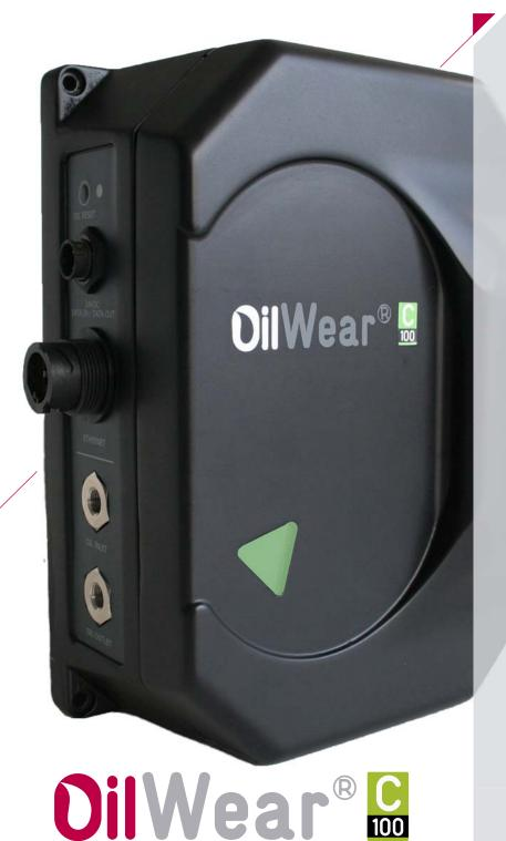
atten2's OilWear® C100 is an online sensor that quantifies particles larger than 4µ present in fluids, and classifies them by size according to ISO, NAS or SAE standards. This is a low cost sensor designed to be permanently installed on a machine, or to be installed on multiple machines, providing real-time information on contamination of fluids.
