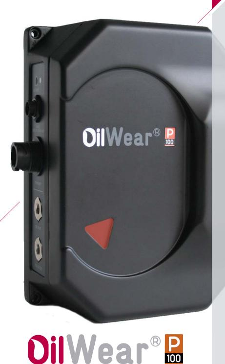
atten2's OilWear® P100 is an online sensor that quantifies particles larger than 14µ present in fluids and classifies them by size in 4 channels. This is a low cost sensor designed to be permanently installed on a machine, or to be installed on multiple machines, providing real-time information on contamination of fluids.
