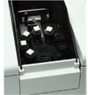
9+1 Cell Changer installed in Lambda 25's sample compartment.
