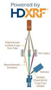
Doubly Curved Crystal (DCC) optics and multiple energy beams reduce background noise and separate coating composition from base material.
