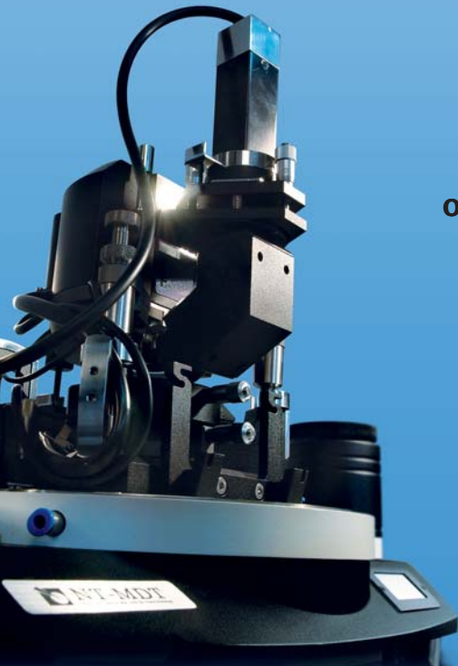
SNOM based on quartz fibers
