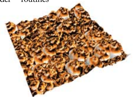
ARgyle Channel Overlay, Second Mode (Dual AC) Amplitude Image of ZnO, 1µm Scan.
