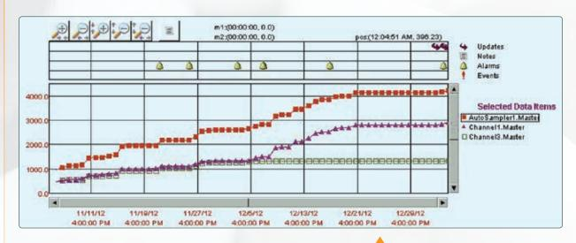
Optional remote monitoring and diagnostic software monitors number of injections and system status in real time
