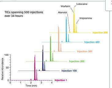
500 injections of four drugs in pooled, crashed human serum demonstrate the Prelude SPLC system's ability to generate reproducible separations in research and toxicology laboratories. Runs were multiplexed using the same TurboFlow and HPLC method on two chromatographic channels and a single mass spectrometer. MS area count RSDs for the 500 runs were <10% for all four compounds. No internal standard was used for normalization.
