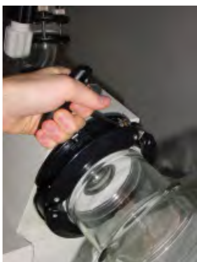
Fig. 4.10: Tightening the snap flange coupling
