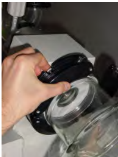
Fig. 4.12: Opening the snap flange coupling
