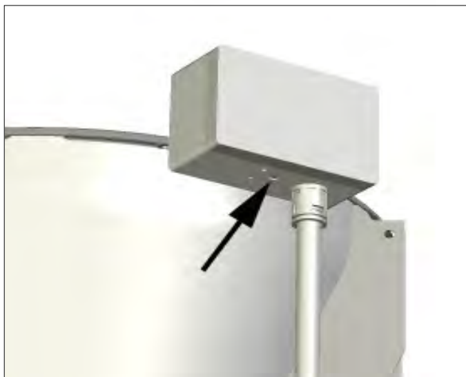
Fig. 5.2: Resetting the over-temperature limiter
