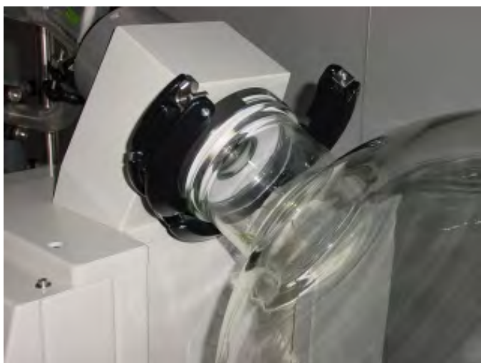
Fig. 4.8: Fitting the flask
