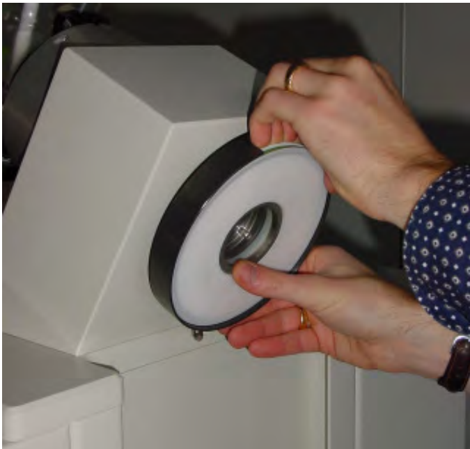
Fig. 6.3: Removing the evaporating flask seal
