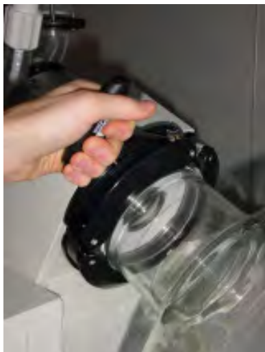
Fig. 4.11: Releasing the snap flange coupling
