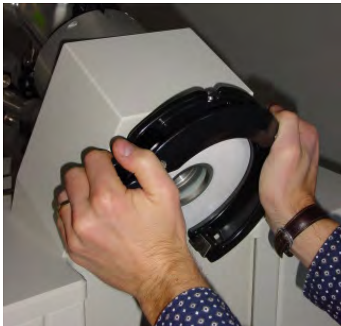
Fig. 6.2: Assembling the snap flange coupling
