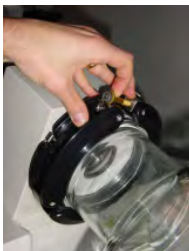
Fig. 4.9: Closing the snap flange coupling
