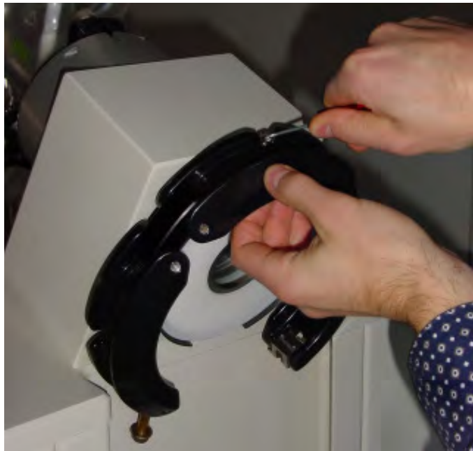
Fig. 6.1: Taking apart the snap flange coupling
