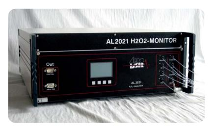
The AL2021 was originally developed for environmental and climate research and is employed worldwide in atmospheric monitoring stations. Since  $H_2O_2$  is getting more and more important in the field of sterilisation and decontamination, the AL2021SC was developed especially for process control during decontamination. It is widely used by the pharmaceutical industry for controlling the atmosphere inside filling systems.
