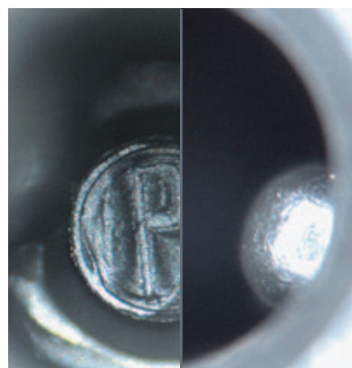
Enlarged detail of an injection nozzle – left: with Leica LED3000 NVI™, right: with conventional ring light
