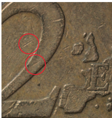
Leica LED3000 MCI™: scratches become visible with the left illuminator arc
