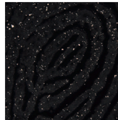
Leica LED5000 MCI™: The same sample in flat incident light. Clearly visible: dust particles
