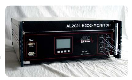
The H<sub>2</sub>O<sub>2</sub> monitor AL2021 from Aero-Laser has an extraordinary high sensitivity and a unique low detection limit of 100ppt (parts per trillion) for gaseous samples and 100 ng/liter (eg.  $2 \times 10^{-9}$  molar) for liquid samples, respectively. The complete chemical processing, including gas stripping, is integrated into the instrument.
