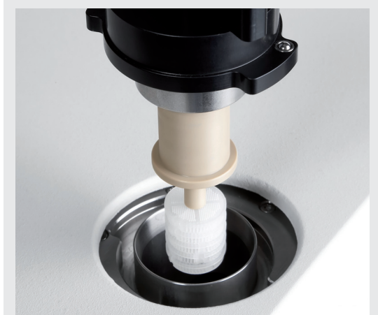
Specimens ready to be inserted into the microwave chamber
