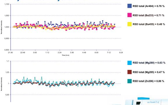
Stability is better than 1% over more than ten hours. This performance allows the analysis of hundreds of samples per day.
