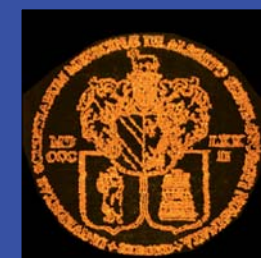
Ultrathin titanium film. AFM nanolithography image obtained by electrical local probe oxidation technique. Scan size 1.9x1.9 \mu\text{m} .
