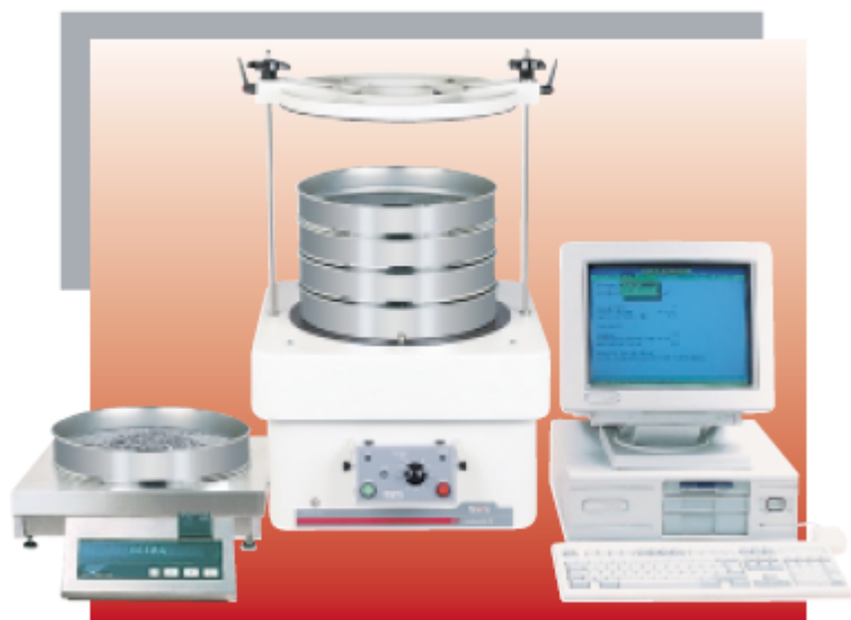
"analysette 18" with computer and balance for automatic sieve evaluation with „autosieve“
