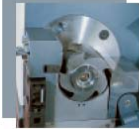
standard rotor with V-cutting edges and fixed knives
