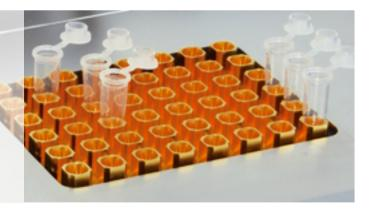
For the SpeedCycler<sup>2</sup> various, interchangable blocks are available. Both, **S**tandard-**P**rofile-**R**apid (SPR) blocks as well as the Low-**P**rofile-**R**apid (LPR) blocks are applicable to the SpeedCycler<sup>2</sup>. Therefore standard PCR consumables can be used as well as the low-profile PCR consumables.
