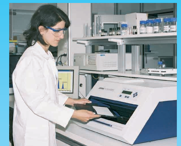
(12) The object, here a 20 × 10 cm HPTLC plate, is positioned on the scanning table and simply inserted. The coordinates are displayed during manual positioning of the stage and can be entered into the program by mouse click.
