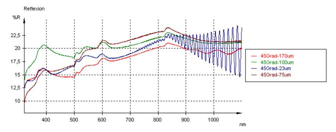
As an example the reflectance spectrum of foil with a film thickness of 23  $\mu$ m was evaluated with a special software for film thickness calculation. As a material plastic with denoted refractive index below and Cauchy-coefficients was selected. Following film thickness was determined:
