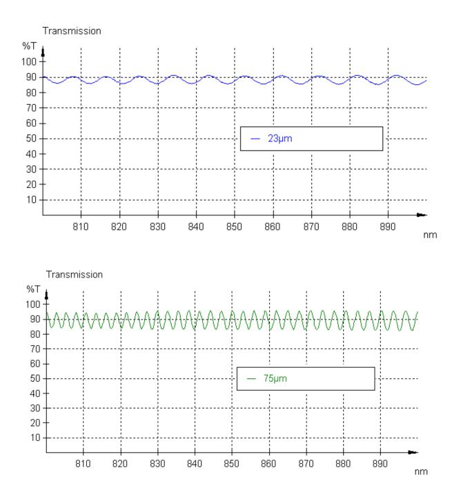
A correlation is clearly indicated between film thickness and transmittance spectra of foil. The distance from maximum to maximum is bigger (ca. 9.2 nm) at foil with smaller film thickness (23  $\mu$ m) and smaller (ca. 1.2 nm) at foil with bigger film thickness (170  $\mu$ m).
