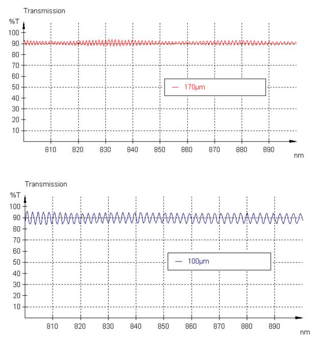
Film thickness and transmittance measurements of foil in SPECORD  $^{\otimes}$  250 Plus Reference: UV\_Plus\_04\_12\_e | 02/ 2012 | ÖZ
