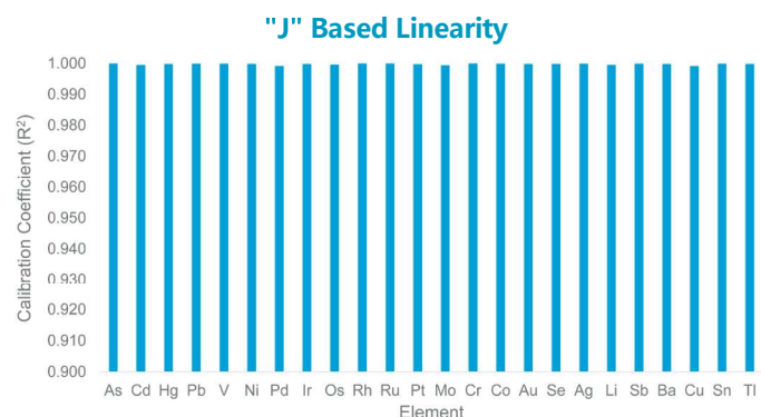
Figure 2. Autocalibrations linearity >0.999 for all class 1, 2A, 2B, and 3 ICH elements.
