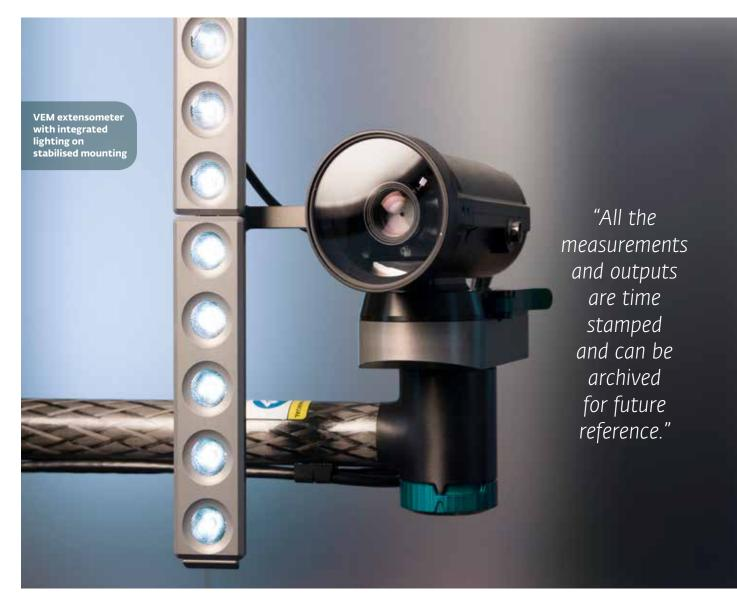
inius Olsen's VEM 100 series of video extensometer modules are designed to measure higher levels of strain (>10%) in tensile, compression, shear and flexural modes. The units are fully integrated with the testing machine and results-reporting software, supporting multiple gauge length click and drag placements, strain rate control and real time results during and throughout the test.
