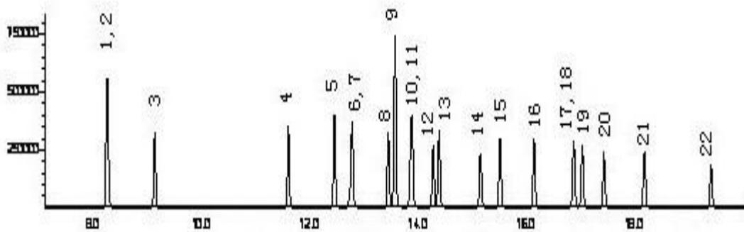
1—PCB28-2',3',5',6'-d<sub>4</sub>; 2—PCB28; 3—PCB52; 4—PCB101; 5—PCB81; 6—PCB77;
