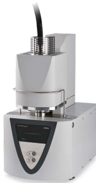
STA 2500 Regulus® with transfer line for STA-FT-IR coupling
