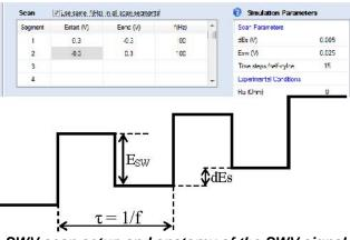
**SWV scan setup and anatomy of the SWV signal** Three parameters define the signal.  $f,dE_s$  and  $E_{sw}$  are available on the setup screen.
