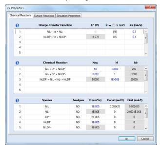
**Typical Parent Setup Screen of an ECE System.** The chemistry and the electrochemistry of the system can be defined through the parent setup screen.
