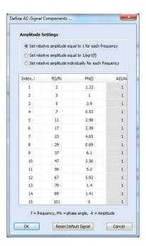
**IMP signal definition** The signal can be defined with up to 15 components with individual frequencies phases and amplitudes. The amplitudes can be fixed to the fundamental amplitude, defined to be  $1 /\sqrt{f} f$ , or adjusted individually.
