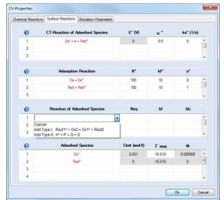
**Surface Reactions Setup Tab** DigiElch 7 can be used to simulate adsorption-desorption and surface reactions with unprecedented detail.
