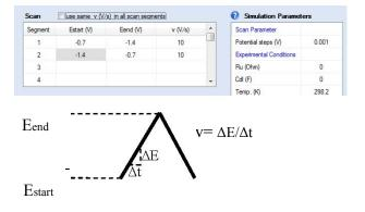
**CV** setup and anatomy of the CV signal Three parameters define the signal.  $E_{\text{start}}$ ,  $E_{\text{end}}$ , and sweep rate are available on the setup screen as shown.
