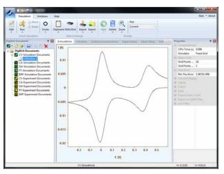
**CV simulations** The simulations can include adsorbed species as well as species diffusing from solution.
