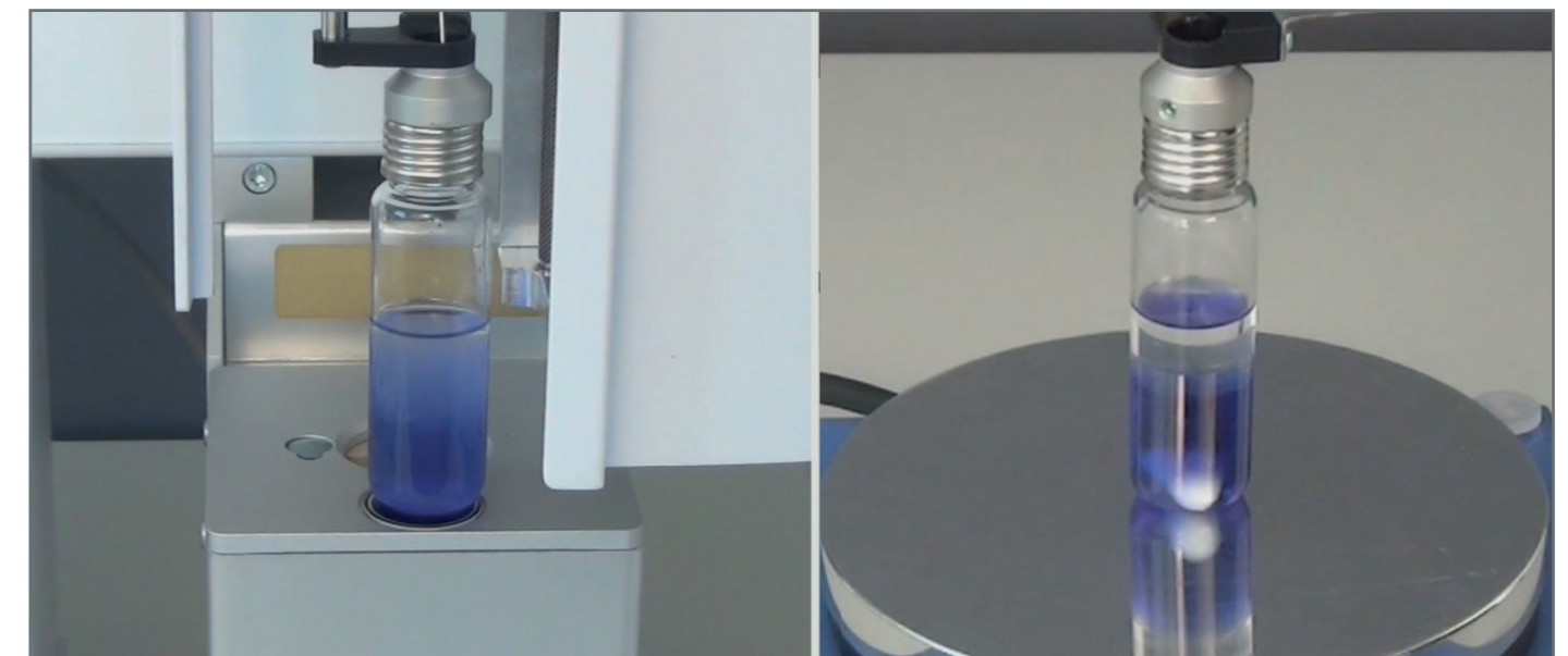
Figure 4: The PAL HeatEx Stirrer (left) gives superior results for liquid/liquid extractions, i.e. smaller droplets and hence more intense exchange between organic and aqueous layer when compared to liquid/liquid extraction with a magnetic stirrer at 1000 rpm (right).
